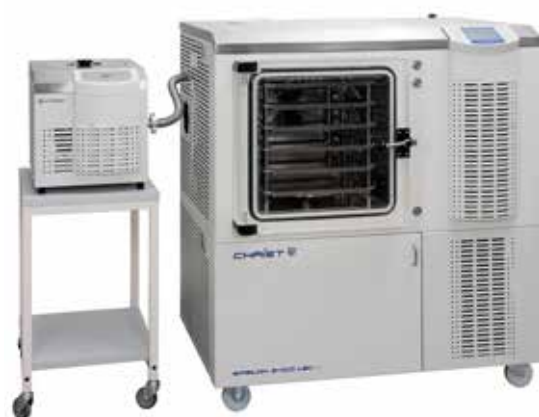
LyoCoN vessel and connected pilot system Epsilon 2-10D LSCplus.
