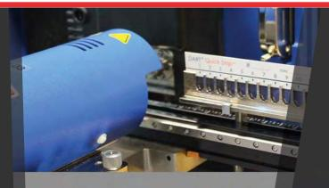
Automated solid and liquid sample presentation system. Utilize our QuickStrip<sup>®</sup> consumables for thermal profiling and comparative sample analysis
