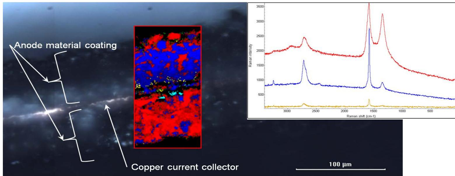
The red color indicates the presence of carbon black while the blue color represents graphite. The distribution of these materials on the two sides of the electrode is significantly different. The copper current collector is in the center.
