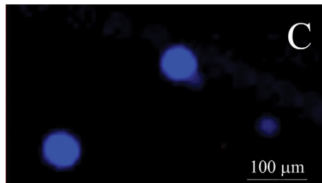
Figure 4: B , distribution of irregular shaped PE particles; C , distribution of PS-DVB; D , distribution of PE-TiO 2 microspheres. Enlargement of specific region of Figure 1 to emphasize the chemical image resolution reachable with 10 micron pixel size.
