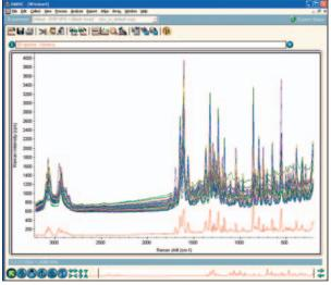
Figure 2: Spectra collected from 25 points on the surface of a scraped painkiller tablet with the VDPS turned off (excitation laser spot size approximately 10  $\mu$ m). The spectrum in red is the variance between the 25 spectra. Spectra collected using 780-nm high-brightness laser and full-range grating on a DXR SmartRaman spectrometer equipped with a UPS accessory with a Well-Plate Autosampler.
