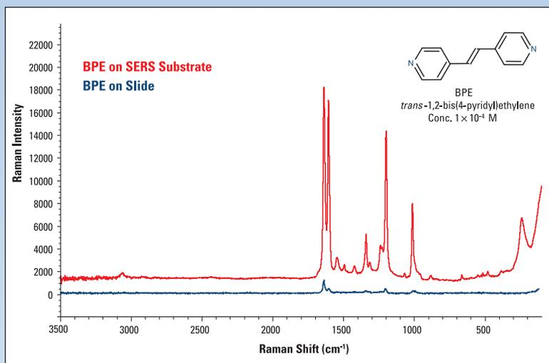
Figure 2: Comparison of Raman spectrum of a BPE solution on a plain surface and on a SERS substrate. The bottom spectrum, in blue, is the Raman spectrum of BPE deposited on a slide and allowed to dry. The top spectrum, in red, is the spectrum of BPE deposited on a SERS substrate and allowed to dry. BPE concentration was 1 × 10<sup>-4</sup> molar, and the data was collected using 780 nm excitation at 1 mW.
