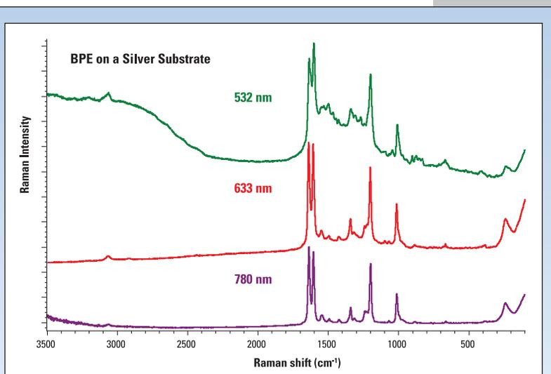
Figure 4: These are the spectra resulting from analyzing the same spot on a silver substrate with BPE on it, using three different lasers, 532, 633, and 780 nm. All the spectra were collected using the same collection conditions: 1 mW laser power at sample, 25 micron slit aperture, and 2 one-second exposures. All spectra are displayed on the same intensity scale, just vertically offset for display purposes.
