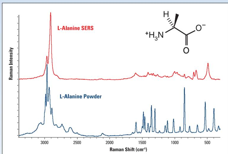
Figure 3: A comparison of l-alanine spectra obtained from bulk powder, shown on the bottom in blue, and from SERS of a dilute solution dried onto a silver SERS substrate, shown on the top in red. Both spectra were obtained using a 633 nm laser. The zwitterion ion form of l-alanine is shown on the top right corner.
