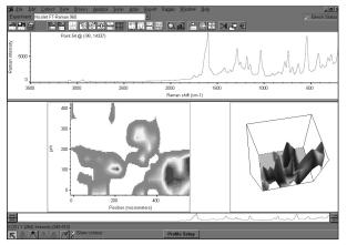
Figure 6: Contour display of the tablet sample mapping data, mapping the peak intensity at the 1042  $\rm cm^{-1}$  band of aspirin
