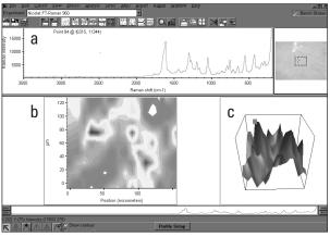
Figure 4: Atlµs<sup>™</sup> software InterLink window provides several views of the sample data. (a) A video image of the sample area shows little detail, while the color contour image (b) and the three dimensional map (c) indicate a small amount of chemical variability across the tablet.
