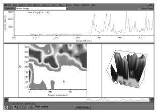
Figure 5: Contour display of the tablet sample mapping data, looking only at the peak intensity of the 857 cm<sup>-1</sup> band of acetaminophen
