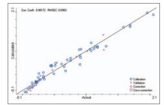
Figure 7: Calibration plot for methanol
