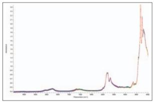
Figure 2: Unprocessed spectra of biodiesel standards
