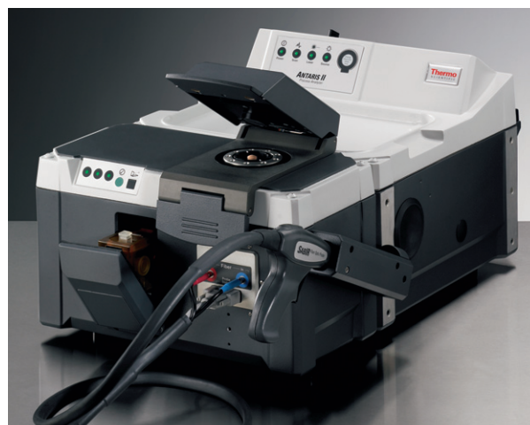
Figure 1: Antaris FT-NIR Method Development System
