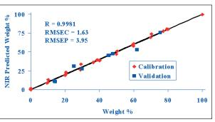
Figure 14: Calibration plot for the quantification of  $\alpha\mbox{-lactose}$  monohydrate in the ternary mixtures
