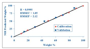
Figure 9: Calibration plot for  $\alpha$ -lactose anhydrous in the binary mixture with amorphous lactose
