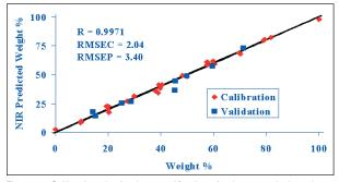
Figure 15: Calibration plot for the quantification of  $\alpha\mbox{-lactose}$  anhydrous in the ternary mixtures
