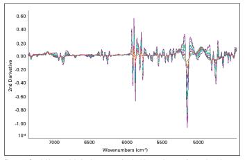
Figure 6: Overlaid second derivative spectra for the binary mixtures of amorphous lactose and  $\alpha$ -lactose monohydrate in the region of interest for calibration (4482 – 7362 cm<sup>-1</sup>)
