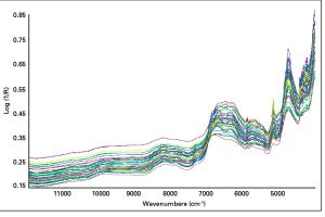
Figure 12: Full-range FT-NIR spectra for the ternary mixtures used in this study
