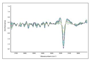
Figure 10: Overlaid second derivative spectra for the binary mixtures of  $\alpha$ -lactose anhydrous and  $\alpha$ -lactose monohydrate in the region of interest for calibration (4902 – 5768 cm<sup>-1</sup>)
