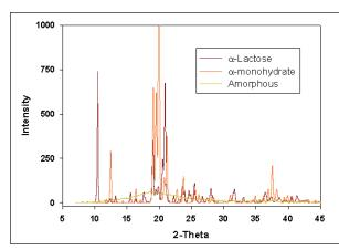
Figure 1: X-ray Powder Diffractograms for all three crystalline forms of lactose used as starting materials for this study
