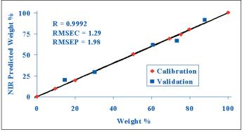
Figure 7: Calibration plot for the  $\alpha\text{-lactose}$  monohydrate in the binary mixture with amorphous lactose
