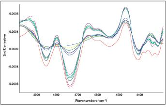
Figure 8: Overlaid second derivative spectra for the binary mixtures of amorphous lactose and  $\alpha$ -lactose anhydrous in the region of interest for calibration (4287 – 4945 cm<sup>-1</sup>)
