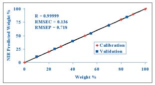
Figure 11: Calibration plot for  $\alpha$ -lactose monohydrate in the binary mixture with  $\alpha$ -lactose anhydrous
