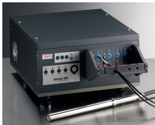
Figure 1: Antaris MX FT-NIR analyzer used for collecting the spectroscopic information from the cell cultures
