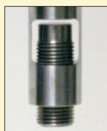
Figure 2: Transfectance probe used in the analysis, showing detail of adjustable pathlength.
