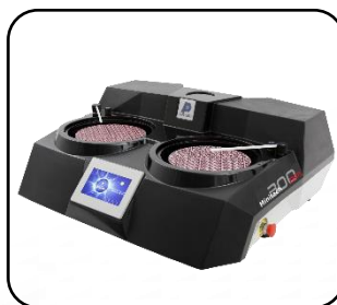
Minitech 250 DP1 2 plates, 1 engine
