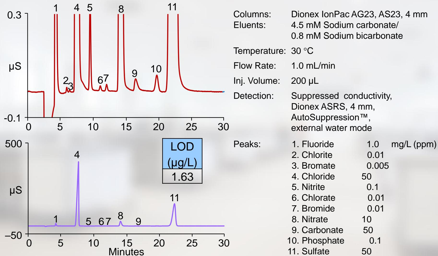
**Recommended carbonate column for EPA Method 300.0 (B)**
