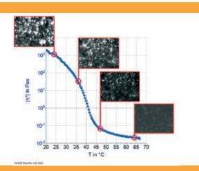
**Rheo-optical investigation of the temperature-dependent crystallization of a crude oil.** The test was performed with the RheoScope module in combination with the active upper-temperature control module and a 60 mm parallel plate measuring geometry.
