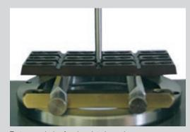
Texture analysis of a chocolate bar using a bending and breaking tool
