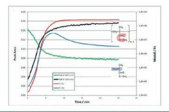
Acrylate glue curing monitored with the Rheonaut module on the HAAKE MARS and Nicolet iS10 FTIR spectrometer. The increase of the sample's moduli (red and blue) corresponds with the decreasing signal of the starting material (monomer in green) and the increasing signal of the final material (polymer's ester bond in black)
