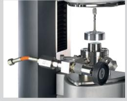
Configuration for high pressure tests
