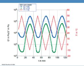
Rheological swing test to predict the temperature stability of cosmetic emulsions (Brummer et al.\*). The test was performed with a 20 mm serrated parallel plate measuring geometry and a peltier temperature control module in combination with an insulated sample cover.
