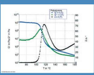
**Dynamic Mechanical Thermal Analysis (DMTA) of a polystyrene.** The test was performed with 8 mm parallel plates measuring geometry and the Controlled Temperature Test Chamber (CTC).
