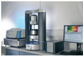
Modular rheometer platform HAAKE MARS with Rheonaut module and Thermo Scientific<sup>™</sup> Nicolet<sup>™</sup> iS<sup>™</sup>10 FT-IR spectrometer
