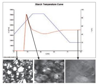
**Temperature ramp study of potato wild type starch in water.** For the measurement the HAAKE MARS was equipped with the RheoScope module including electrical temperature control and a 35 mm parallel plates geometry.
