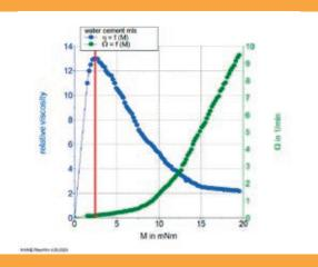
**Determination of yield stress in Controlled Stress (CS) mode of a cementitious paste.** For the measurement the HAAKE MARS was equipped with the measuring cell for building materials and a FL26 CMC vane type rotor.
