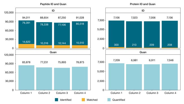
Reproducible identification and quantification using PepMap Neo columns: HeLa peptides and proteins over four EASY-Spray PepMap Neo columns (17497583, 75 µm I.D. × 750 mm) while using the Vanquish Neo UHPLC system (direct injection workflow) coupled with the Thermo Scientific™ Oribtrap™ Exploris 480 Mass Spectrometer. The reproducibility of these columns has been reported in Thermo Scientific Technical Note (TN74152).
