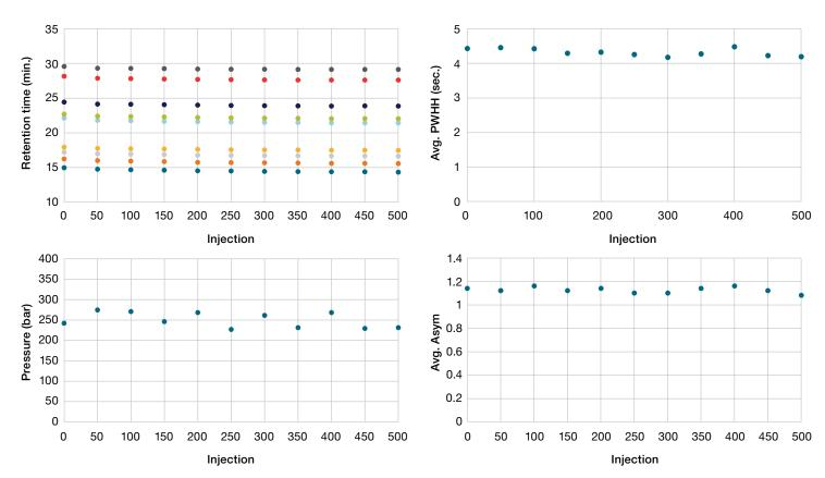
PepMap Neo columns (17487583, 75 µm I.D. × 500 mm) offer excellent robustness: Column ruggedness test from 500 injections with the direct injection workflow using 200 ng HeLa digest. The data shows consistent peak retention time, peak width, peak symmetry, and system pressure.
