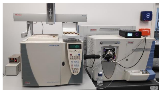
Figure 1: SICRIT® cold-plasma ion source features soft ionization GC-HRMS coupling (Thermo LTQ Orbitrap XL)
