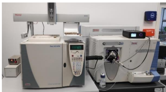
Figure 1: SICRIT® coupling of a Thermo Trace GC Ultra to a Thermo LTQ Orbitrap XL.
