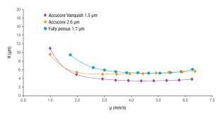
Accucore Vanguish UHPLC columns are more efficient at optimum flow than sub-2 μm fully porous and 2.6 μm solid core columns. Efficiency is maintained over a wider linear velocity range.
