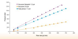
Accucore Vanguish UHPLC columns achieve their efficiency without excessive backpressure.
