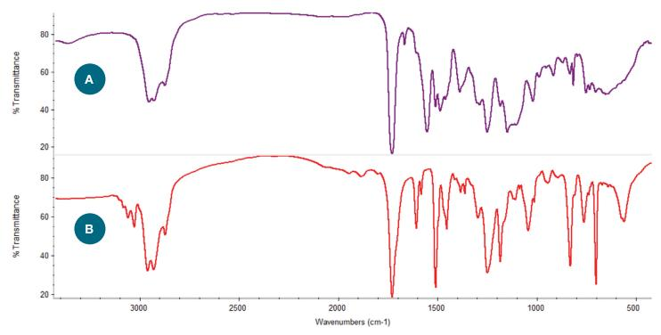
A shows spectrum taken from the outer coating of the soda can, which includes design pigments.B shows spectrum of inner coating of soda can used to protect soda from aluminum can.
