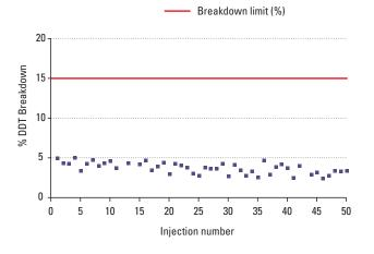
Figure 2: Compound degradation after 50 injections - LinerGOLD exhibits minimal breakdown
