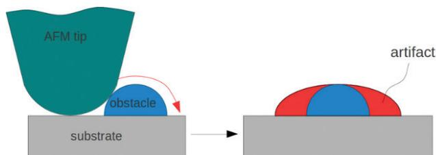
Figure 3. Illustration of the “tip broadening effect” in AFM creating artifacts of wider particle dimensions than truly exist. [3]
