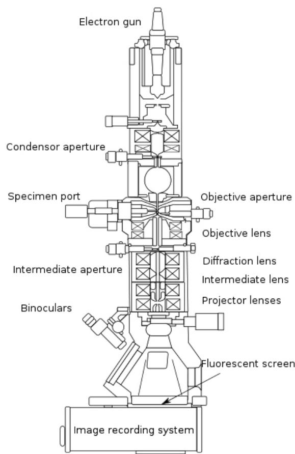
Figure 1. Illustration of how a TEM is constructed [1].
