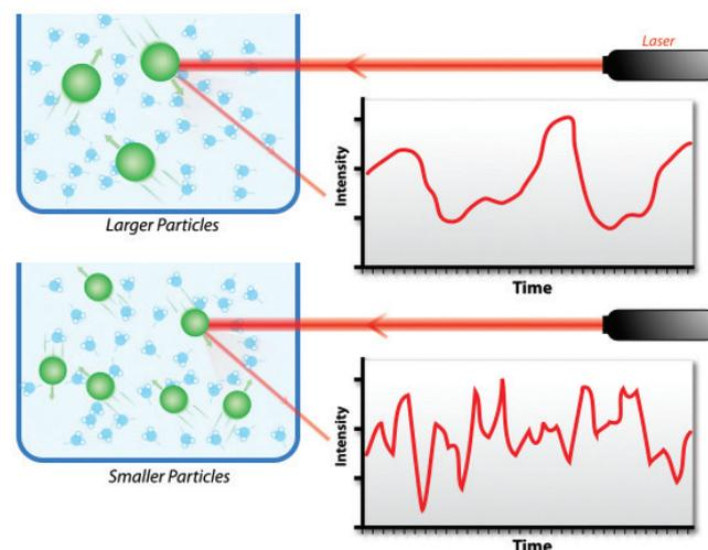
Figure 2. Basic structure of a DLS measurement and example of how particle size influences data observed. [2]
