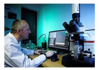
Figure 1. NRC-BRI technical officer Sabahudin Hrapovic uses a LVEM 5 benchtop transmission electron microscope to observe the size and distribution of nanocrystalline cellulose particles.
