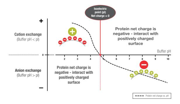
In the fast-paced drug development environment, a platform method to accommodate the majority of mAb analyses is desired. Considerable method development is required to optimize the salt gradient for charge variant separation of each mAb. Ion exchange separations by pH gradient provide the advantage of a generic platform approach, thus saving time on method development. As well, heavy salts are removed from LC systems, resulting in less cleaning and downtime.
