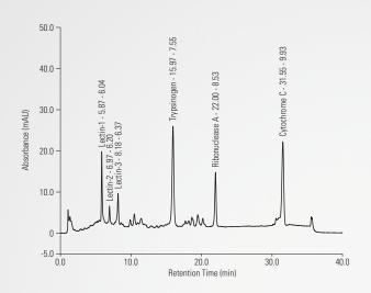
Column: MAbPac SCX-10, 10 μm 4.0 × 250 mm Format: Mobile phase A: 1X CX-1 pH gradient buffer A, pH 5.6 Mobile phase B: 1X CX-1 pH gradient buffer B, pH 10.2 pH gradient: %A %B 0.0 100 0 1.0 100 0 0 31.0 100 34.0 0 100 34.1 100 0 0 40.0 100 Flow rate: 1.0 mL/min Inj. volume: 5 μL 30 °C Temp.: UV, 280 nm Detection: Sample: Protein standard
