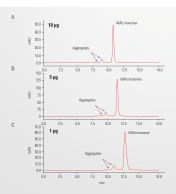
Column: MAbPac SEC-1, 5 um. Format: a 78 × 300 mm b.  $4.0 \times 300 \text{ mm}$ a. 2.1 × 300 mm 50 mM sodium phosphate pH 6.8, Mobile phase: in 300 mM sodium chloride a. 760 µL/min Flow rate: b. 200 μL/min c. 50 µL/min a. 10 µL Inj. volume: b. 5 μL a. 1 µL Temp.: 30°C 280 nm Detection: MAb (1 mg/mL) Sample:
