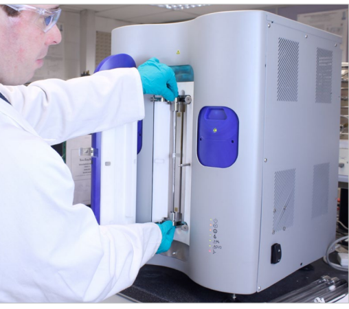
iGC-SEA straight column design - simple sample packing and column loading
