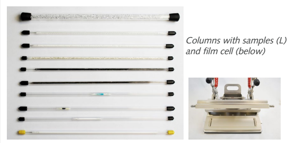
iGC-SEA straight column design - simple sample packing and column loading
