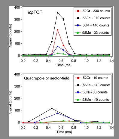
Nanosteel nanoparticles composed of Fe, Cr, Ni, Mo were diluted with milliQ water and measured with the *icp*TOF using H2 in the Q-cell at 3 ml/min to remove ArO interference on 56Fe.
