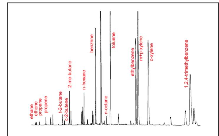
Extended HC analysis on FID (emission gas sample; He or H<sub>2</sub> carrier gas)
