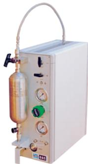
Pressure facility for liquid LPG injection
