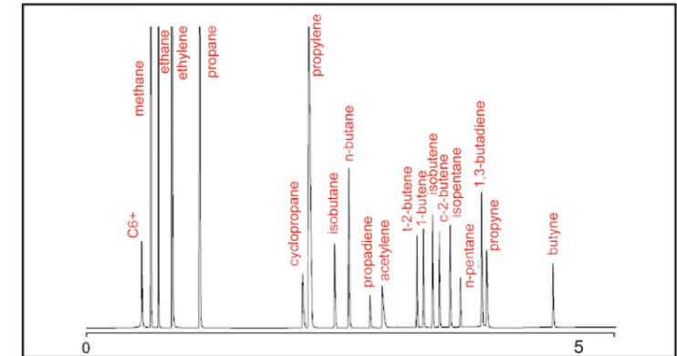
Channel 3: C1-C6 hydrocarbons on FID (He or H<sub>2</sub> carrier gas)
