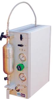
Pressure facility for liquid LPG injection
