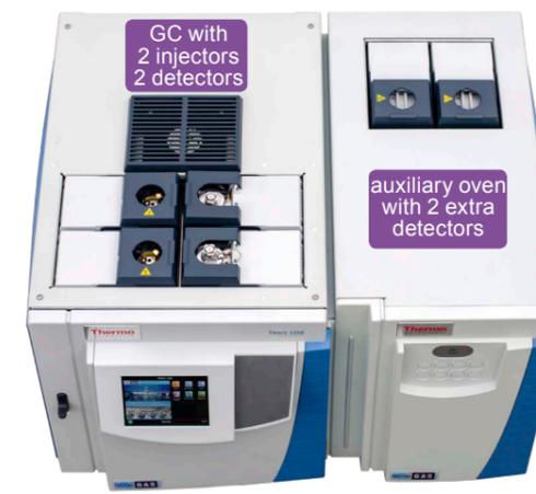
Versatile instrument with large, highly accessible auxiliary oven and InstantConnect injector / detector modules
