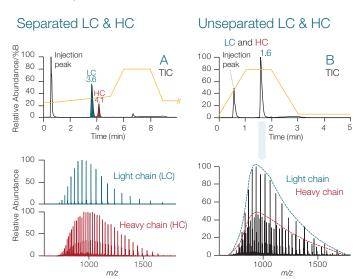
Speed and sensitivity support superb quality detection of antibody light and heavy chains (A), even without chromatographic separation (B). The Q Exactive HF-X MS produces distinct, high-quality baseline-resolved spectra of antibody subunits with superior quality.
