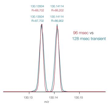
Improved TMT Performance. An MS² spectrum showing baseline resolution of TMT10-130N and TMT10-130C reporter ions. A dedicated TMT scan mode enables the Q Exactive HF-X MS to effectively resolve TMT reporter ions in only 96 msec versus the previous 128 msec method. This assures accurate quantitative results and allows more scans per run for deeper levels of analysis.
