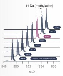
With improved ion transmission provided by the Advanced Quadrupole Technology, it is now possible to efficiently enrich for individual isobaric protein forms for a subsequent top-down analysis.
