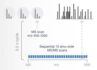
DIA acquisition was performed using a 120,000 FWHM resolution MS scan followed by 15 amu-wide MS/MS windows at 30,000 FWHM resolution with 60 ms maximum injection time.
