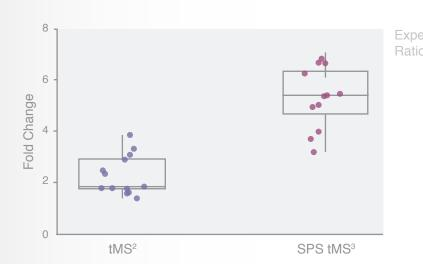
Comparison of results for the TMT tMS² and TMT SPS tMS³ quantification methods shows improved accuracy of the tMS³ method. Each point represents the fold change of a single quantification event for each of the targeted peptides present at 100 amol level in matrix. The expected ratio is 8:1.
