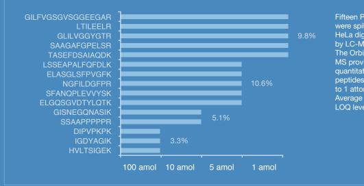
Fifteen PRTC peptides were spiked into 200 ng of HeLa digest and analyzed by LC-MS (30 min run). The Orbitrap Fusion Lumos MS provides accurate quantitation of all 15 PRTC peptides with some down to 1 attomole levels. Average CV% for each LOQ level is shown.
