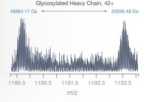
Isotopic resolution of light chain (top panel), and heavy chain (bottom panel), showing the detection of glycosylated forms.
