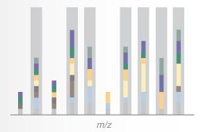
CID MS² spectrum of native peptide target contains multiplexed fragments. Gray bars indicate the predicted fragment target ions that are selected for the following SPS tMS³ step.
