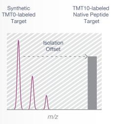
The synthetic TMT0-labeled peptide is detected in the full MS scan. The native TMT10-labeled peptides are isolated by using an offset (*m/z* difference between TMT0 and TMT10).
