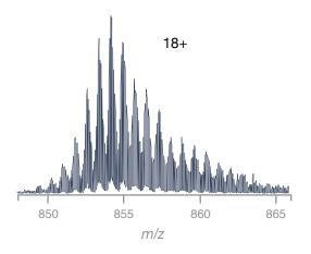
Advanced Vacuum Technology increases ion transmission, improving the quality of intact protein spectra acquired in the high resolution accurate mass Orbitrap analyzer.
