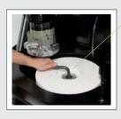
Fast and easy replacement of the grinding wheel
