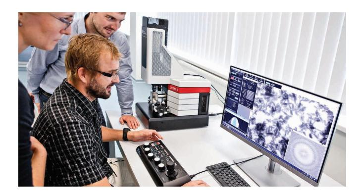
The LVEM 5 seamlessly combines 4 different imaging functionalities into one benchtop instrument, so samples no longer need to be displaced from one microscope to another. Furthermore, switching between imaging modes is easy, with the click of a button the same area of interest of a sample can be imaged in TEM, SEM and STEM modes.
