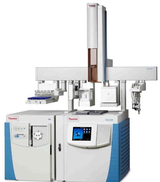
Trace 1310 GC with ISQ Mass Spectrometer and RSH autosampler
