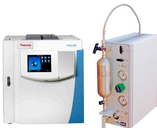
Trace 1310 GC with optional Pressure Facility for injection of Liquefied Gas
