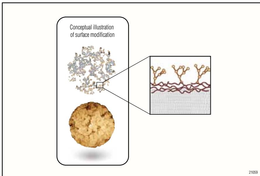
Figure 1. Structure of an IonPac AS20 packing particle.
