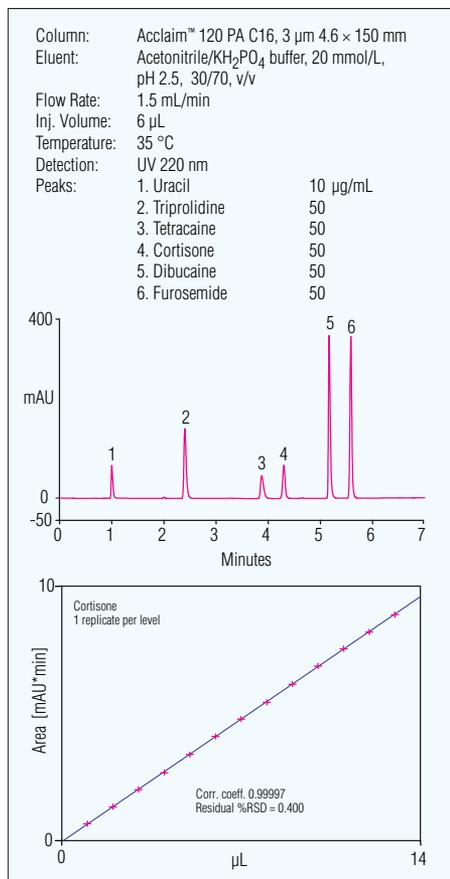
Injector linearity example with partial loop injections (1–13 μL).
