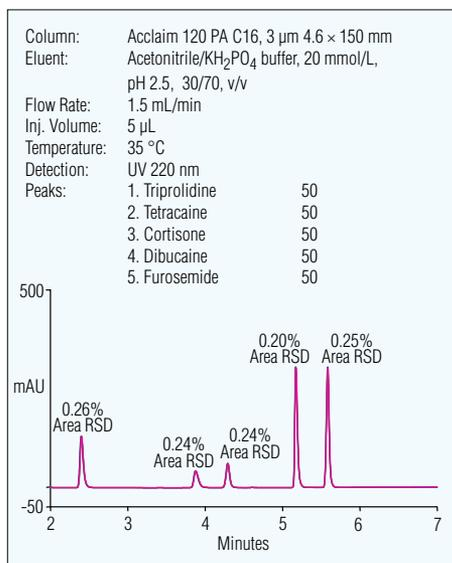
Overlay of six consecutive injections with 5 μL sample volume, using the ACC-3000 with pulled loop technique and UV detection at 220 nm. The typical peak area RSD is <0.3% in partial loop mode.
