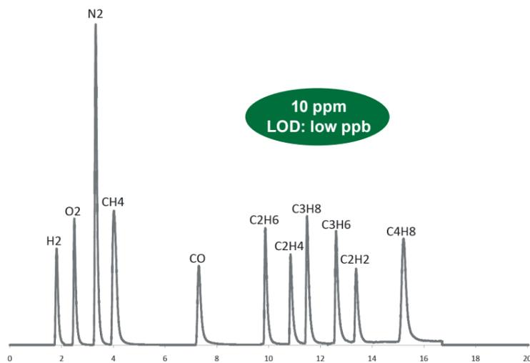
Chromatogram 1: permanent gases and light hydrocarbons, 10 ppm level
