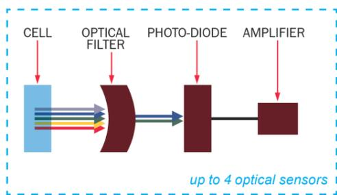
Diagram 1: Plasma Emission Detector, principle
