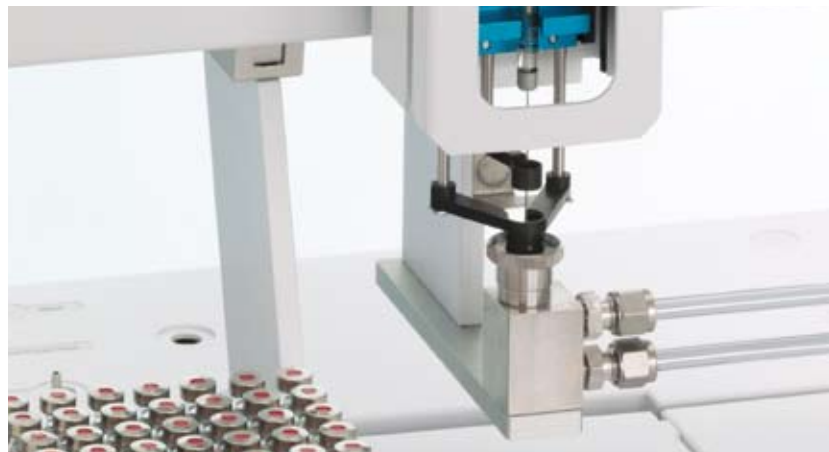
Flow-Through Cell for online analysis
