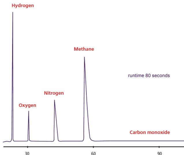
Chromatogram 4. Extended Biogas analysis. CompactGC<sup>4.0</sup>-TCD
