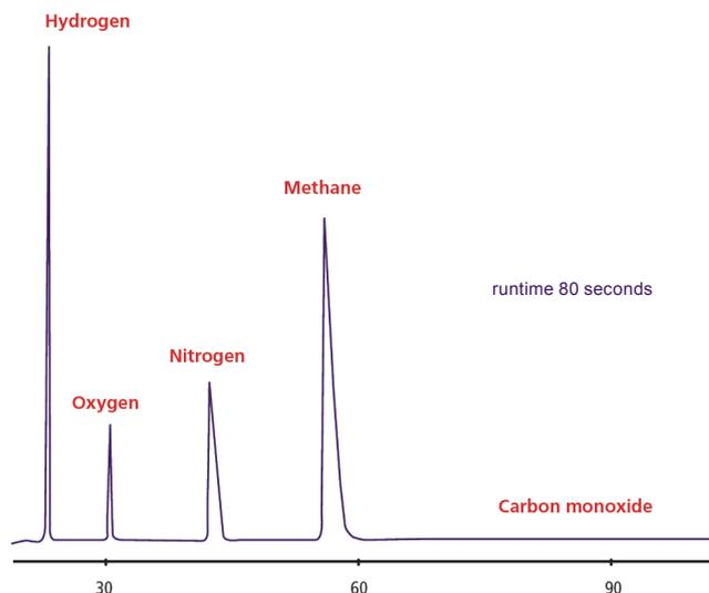
Chromatogram 4. Extended Biogas analysis. CompactGC<sup>4.0</sup>-TCD
