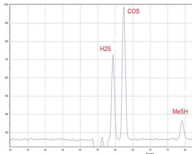
Chromatogram 5: 0.8 ppm H<sub>2</sub>S, 1.3 ppm COS and 350 ppb MeSH in Biogas
