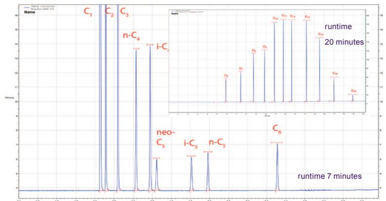
Chromatogram 2. Extended Biogas analysis, GC Trace 1300-FID
