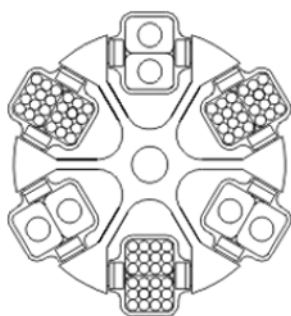
Fig. 15: Permissible and impermissible loading of a swing-out rotor with vessels of various sizes (example illustration)
