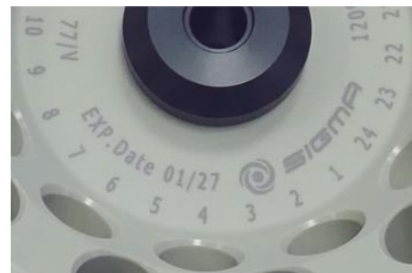
Fig. 7: Different service life – engraving on the bucket/rotor
