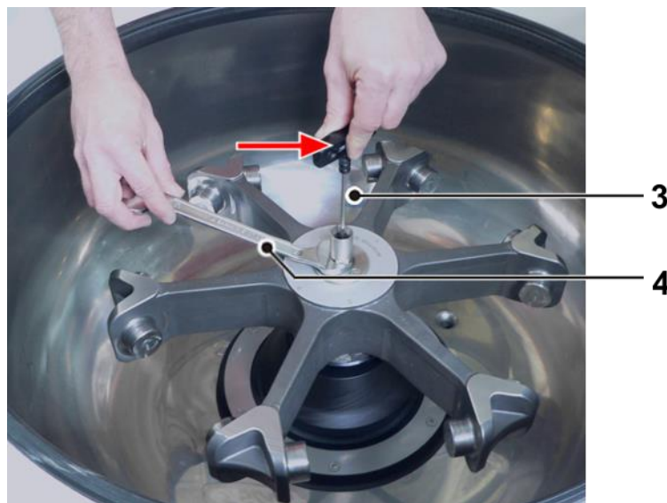
Fig. 13: "Two-finger-principle" for holding the hexagon key
