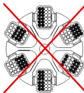
Fig. 16: Permissible and impermissible loading of an angle rotor and a swing-out rotor (example illustration)
