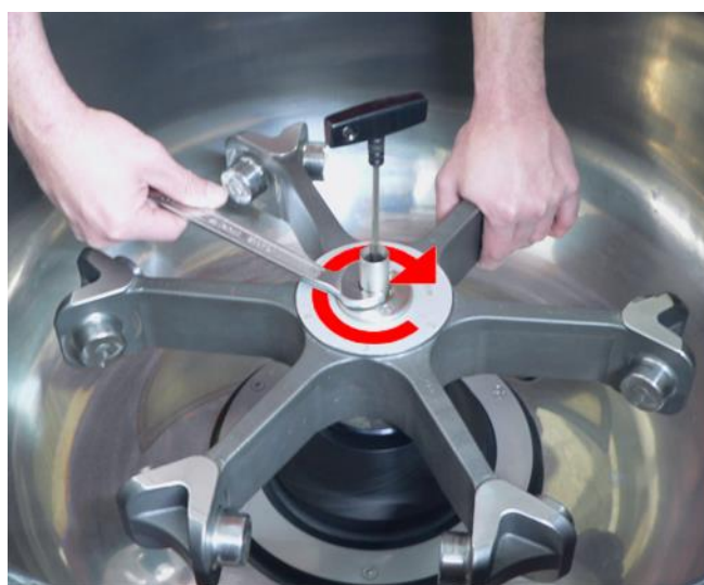
Fig. 14: Fastening of the rotor
