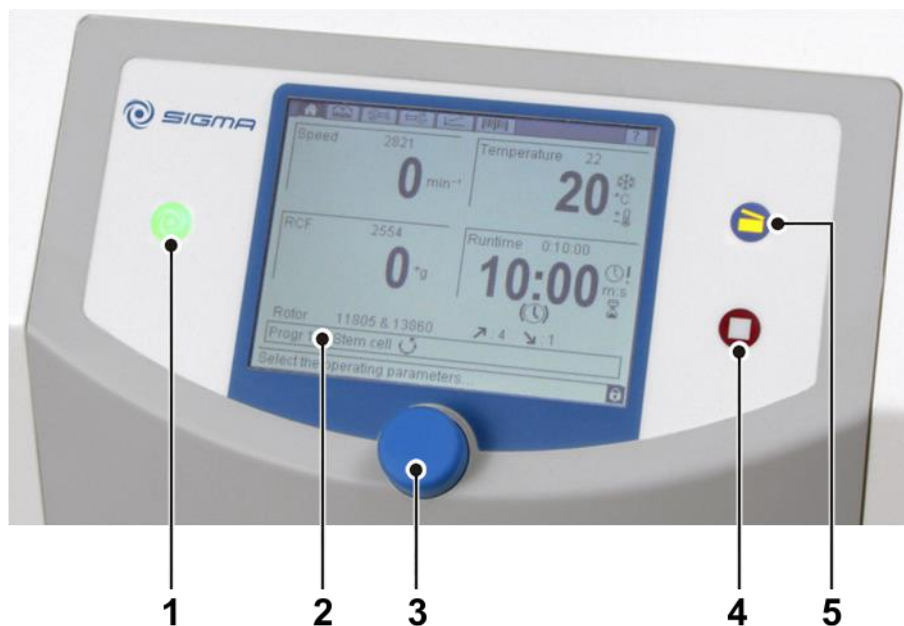
Fig. 19: User interface of the Spincontrol S control system
