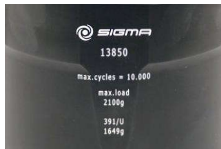
Fig. 5: Different service life – engraving on the bucket/rotor
