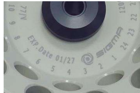
Fig. 5: Different service life – engraving on the bucket/rotor
