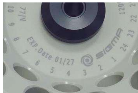
Fig. 6: Different service life – engraving on the bucket/rotor
