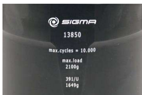
Fig. 6: Different service life – engraving on the bucket/rotor
