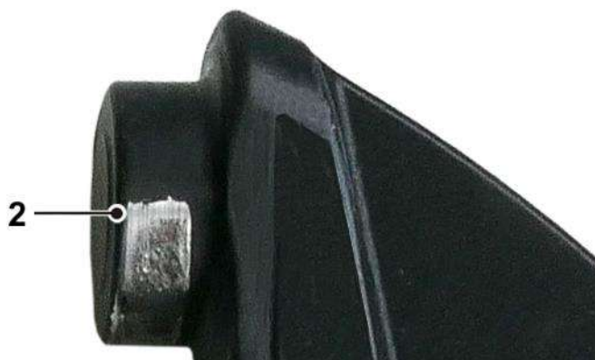
Fig. 8: Load-bearing bolt with completely worn-off coating – greasing required
