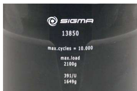
Fig. 5: Different service life – engraving on the bucket/rotor
