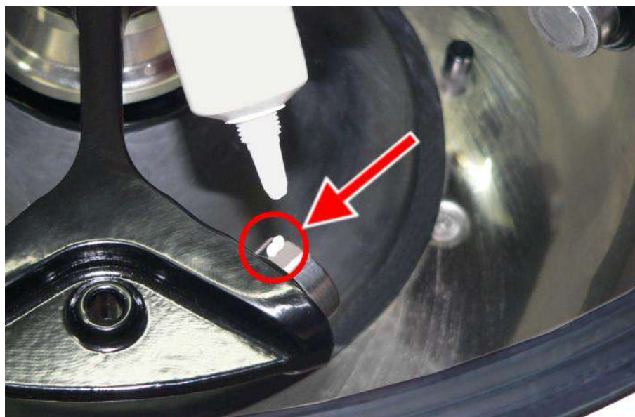
Fig. 37: Sufficient quantity of grease for one bolt
