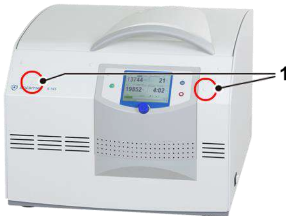
Fig. 35: Position of the openings for the emergency lid release
