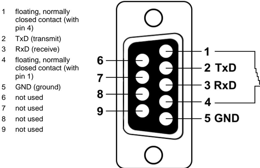
Fig. 5: Pin assignment of the serial interface
