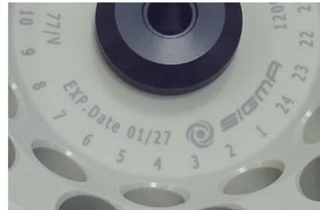
Fig. 7: Different service life – engraving on the bucket/rotor
