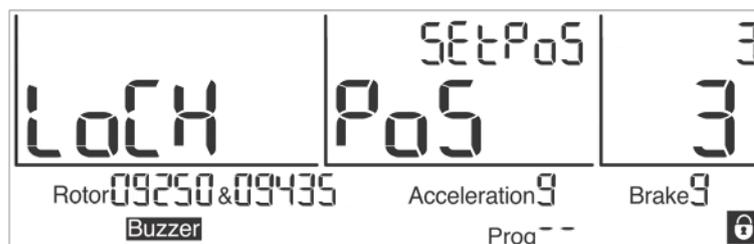
Fig. 34: Indication after the completion of the positioning process
