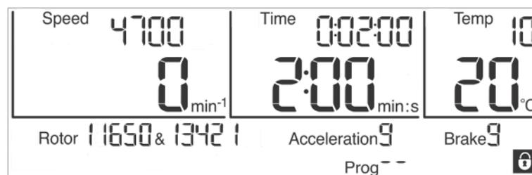
Fig. 29: "Padlock" symbol indicating an activated input lock
