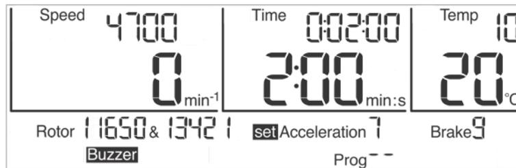
Fig. 25: Preselection of a curve; here: preselection of an acceleration curve
