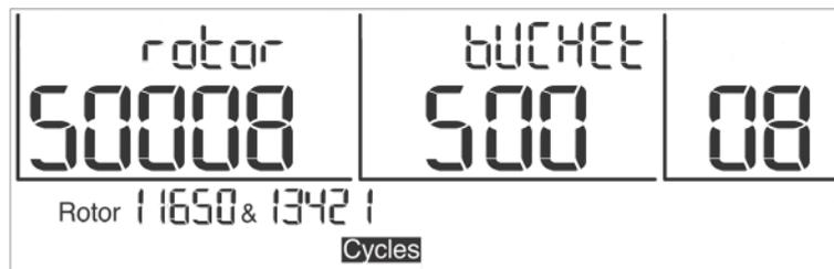
Fig. 28: Display when the maximum number of cycles is reached (flashing)
