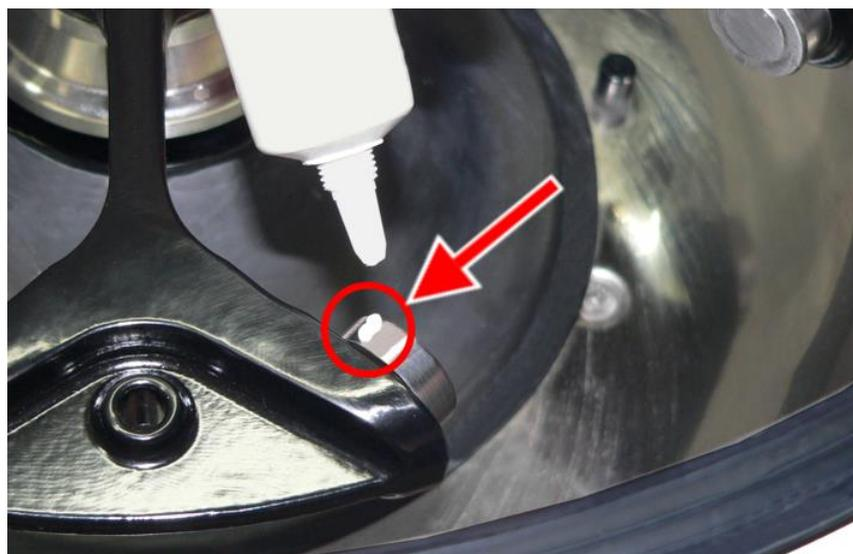
*Fig. 36: Sufficient quantity of grease for one bolt*
