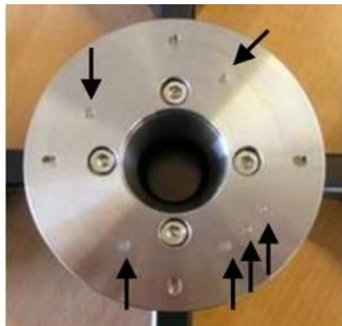
Fig. 32: Magnets on the bottom surface of the rotor
