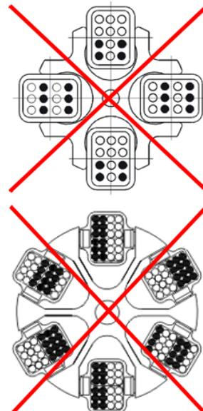
Fig. 14: Permissible and impermissible loading of a swing-out rotor (example illustrations)
