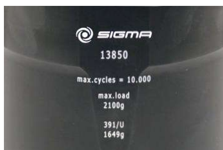
Fig. 5: Different service life – engraving on the bucket/rotor
