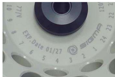
Fig. 5: Different service life – engraving on the bucket/rotor
