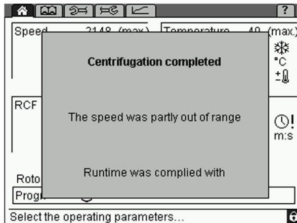
Fig. 22: Example of a centrifugation monitoring message
