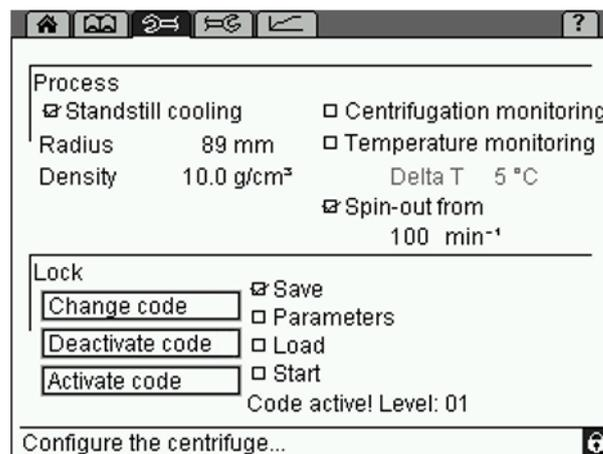
Fig. 23: "Parameters" menu with an active lock (level 01)
