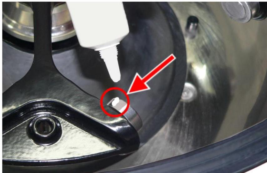
*Fig. 34: Sufficient quantity of grease for one bolt*
