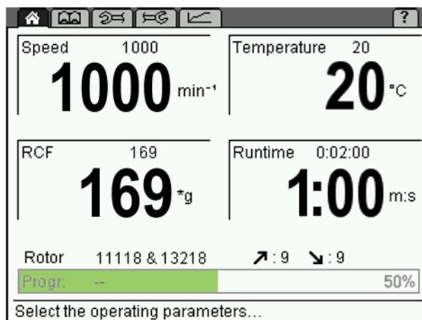
Fig. 19: Progress indicator during a centrifugation run
