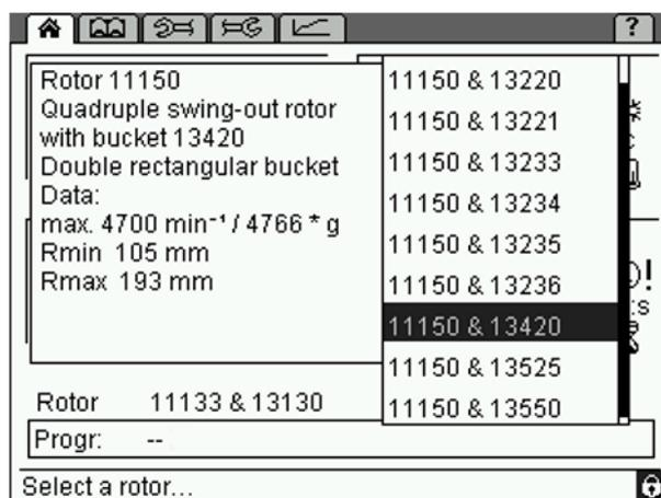
Fig. 16: Rotor selection list, here with potential rotor-bucket combinations and additional information
