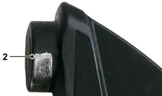
*Fig. 7: Load-bearing bolt with completely worn-off coating – greasing required*
