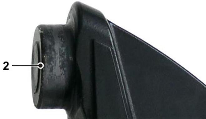
*Fig. 6: Load-bearing bolt with traces of use – no greasing required*
