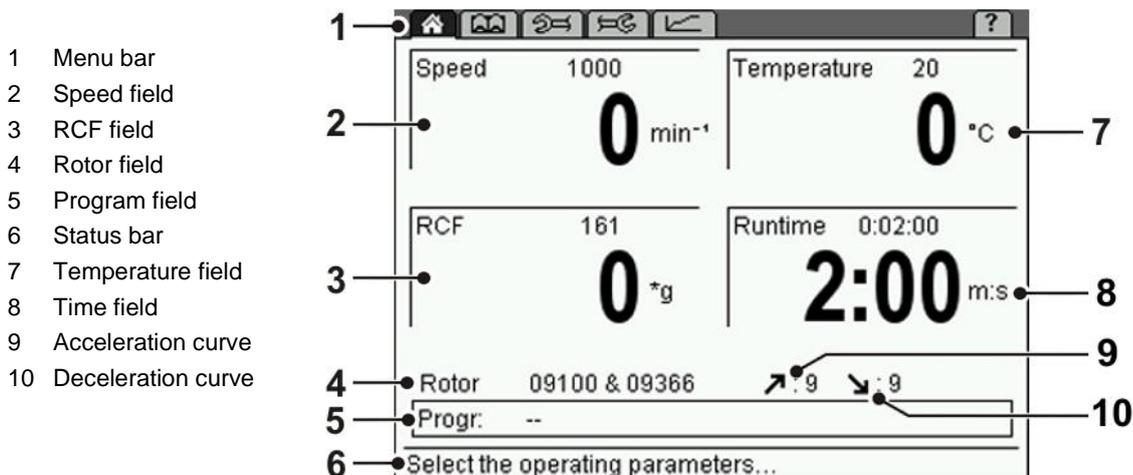
Fig. 14: Display of the Spincontrol S control system
