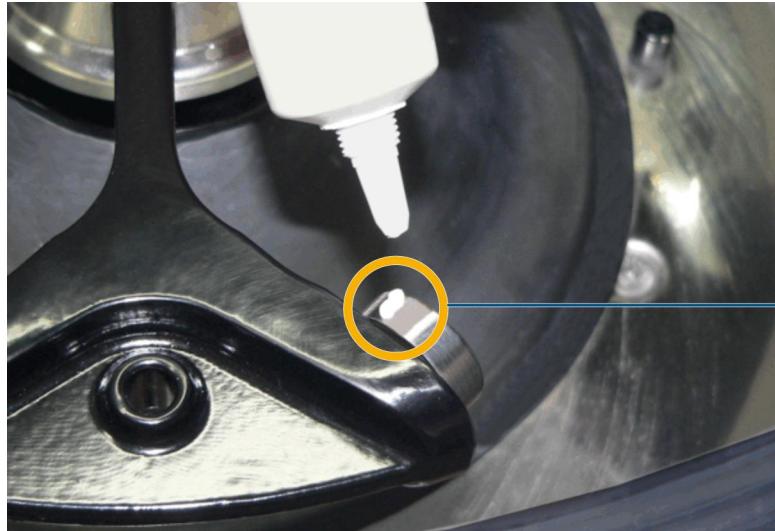
Fig. 59: Applying the grease for load-bearing bolts
