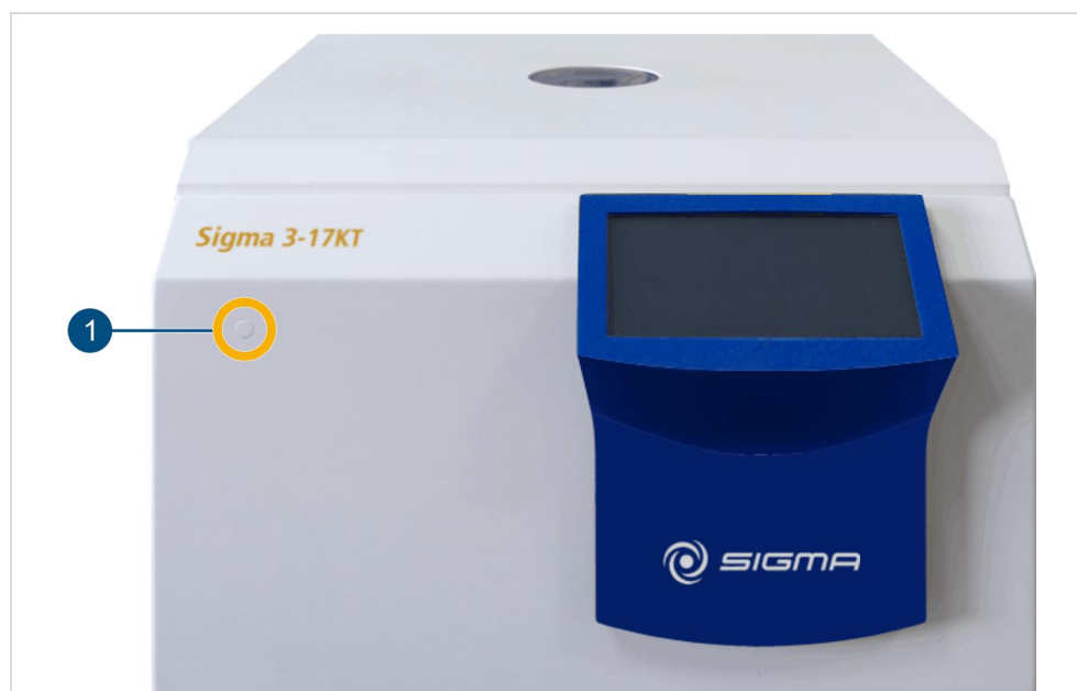
Fig. 62: Position of the opening for the emergency lid release
