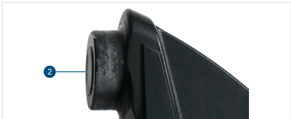
Fig. 57: Load-bearing bolt with traces of use – no greasing required
