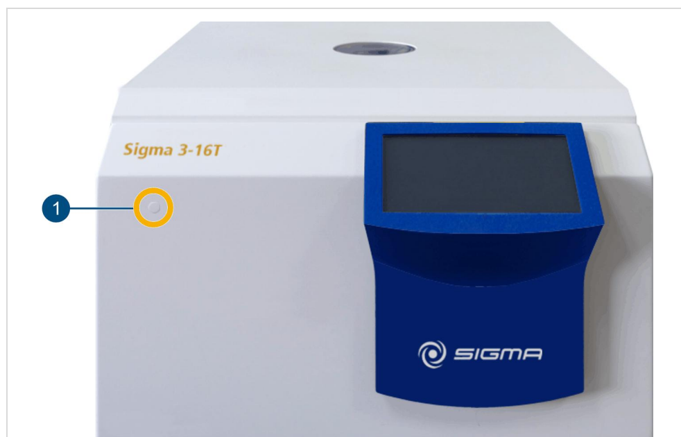
Fig. 56: Position of the opening for the emergency lid release
