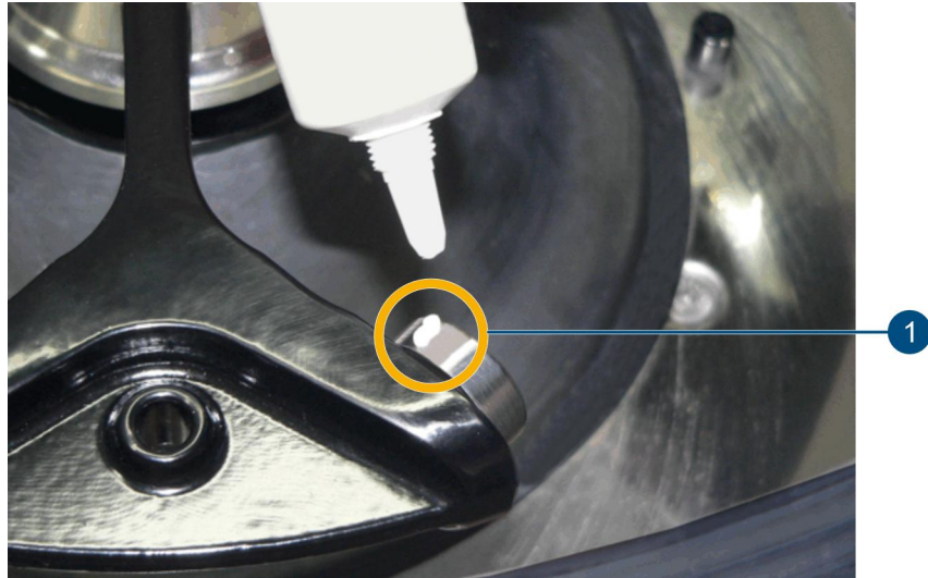
Fig. 53: Applying the grease for load-bearing bolts
