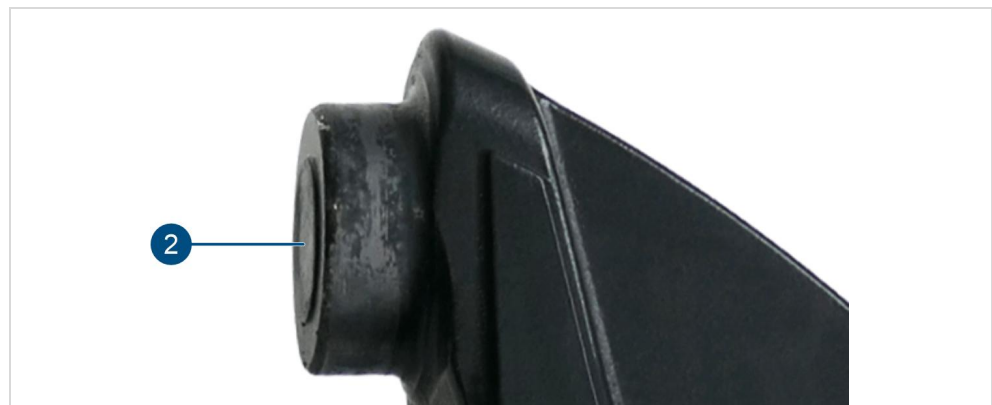
Fig. 51: Load-bearing bolt with traces of use – no greasing required
