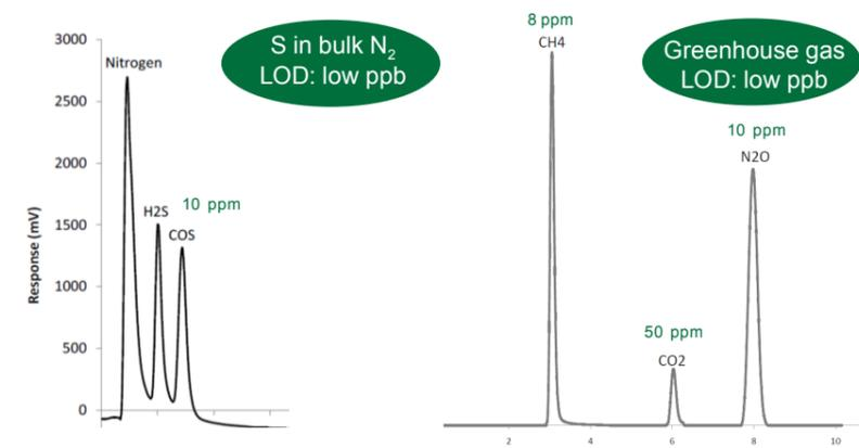
chromatogram 2,3 : sulfur and greenhouse gases
