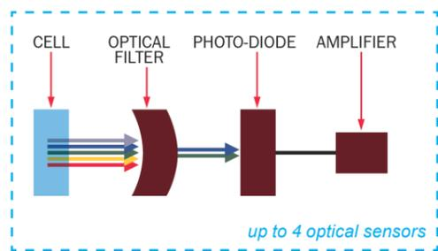
Diagram 1: Plasma Emission Detector, principle
