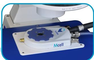
**The GenRH-Mcell** connects to the GenRH-A and is mounted onto microscope platforms. In this way, samples can be observed under precisely controlled ambient humidities.
