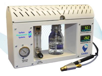
The GenRH-A is the world's most flexible instrument for relative humidity (RH) generation, easily coupling to your characterization systems to deliver precision RH levels from 0 to 98% at ambient room temperatures with ±0.7%RH control.
